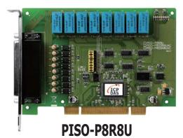
Universal PCI, 8-ch Optically Isolated Digital Input and 8 Relay Output Board
